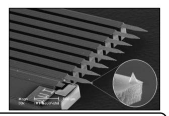
The eight tiny probe tips on the Atomic Force Microscope (AFM) built into NASA's Phoenix Mars Lander. The tip enlarged in the circle is the same size as a smoke particle at its base (2 microns). Photo by courtesy of NASA Jet Propulsion Laboratory (NASA-JPL).
